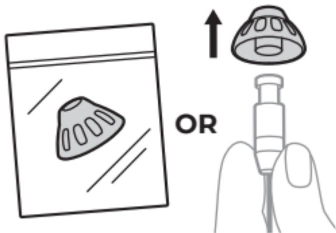
Get a dome for the new receiver wire. Either pick your size from a dome kit (available separately) or firmly pull the dome off of the old receiver wire.
