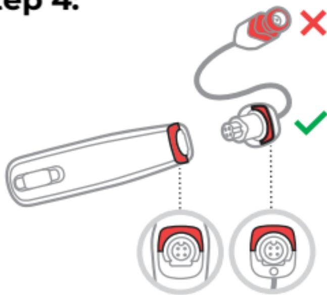
Align the clear plastic end of the new receiver wire with the port on the hearing aid body so the red or blue marks line up.
