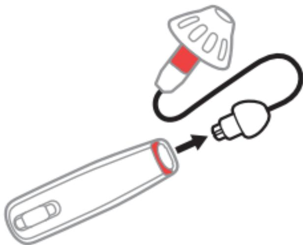
Firmly pull the old receiver wire until it detaches from the hearing aid body.
