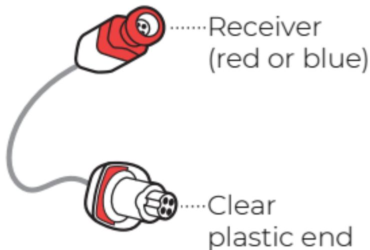
Identify the two ends of the receiver wire.
