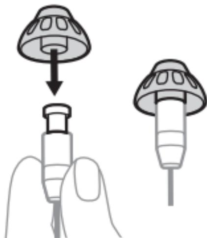
On the new receiver wire, align the opening of the dome with the receiver and slide the dome onto the receiver.
