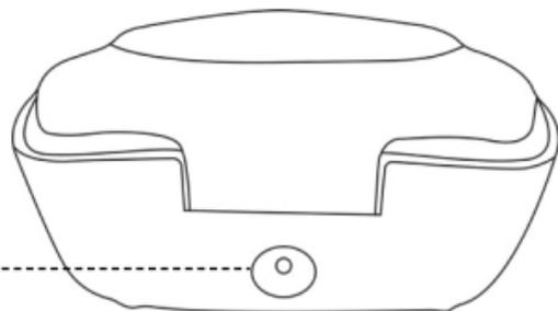
1. Insert the USB cable into the 5V power adapter. Plug the connector into the socket on the rear side of your dryer.
